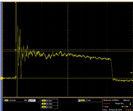
Figure 13: AQHV15 +8kV Contact ESD Clamping Voltage
