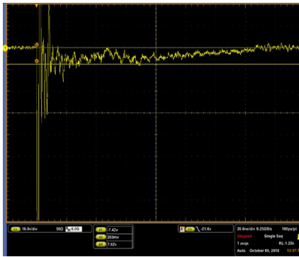
Figure 16: AQHV24 -8kV Contact ESD Clamping Voltage
